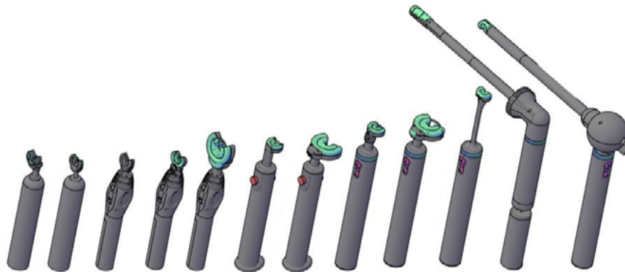
Consecutive iterations of Suttrue , an automated surgical suturing device prototyped on Formlabs SLA printers.
