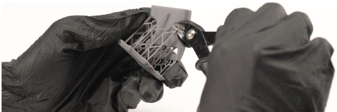
Remove supports with flush cutters, and sand away the remaining support marks for a clean finish.
