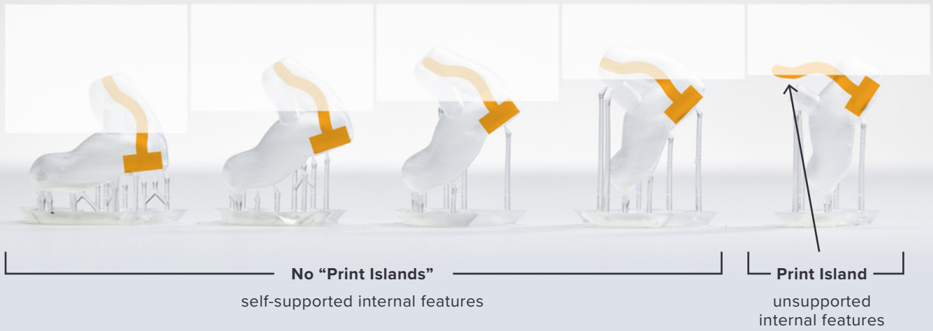
Fig. 10: Each of these five prints are the same, but the orientation can determine the print success. The four prints on the left will print without issue, but the fifth print is oriented in such a way that the internal feature creates a print island.
