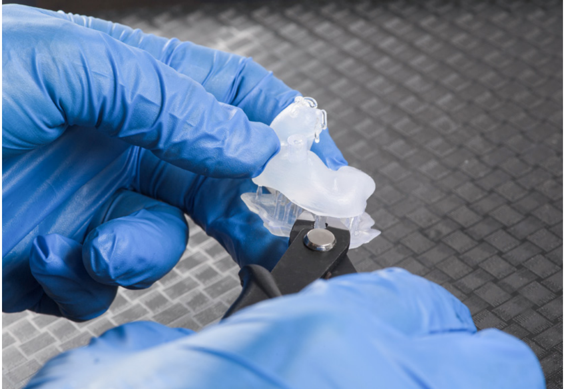
Fig. 18: Removing supports using flush cutters
