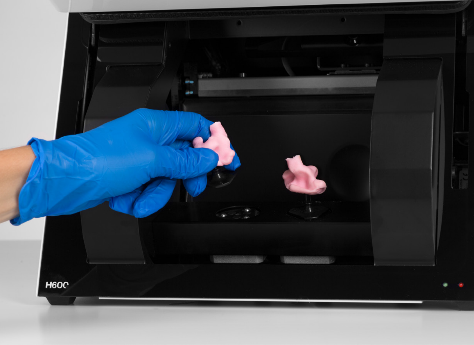
Fig. 5: Scanning the ear impressions using a 3Shape H600 scanner.
