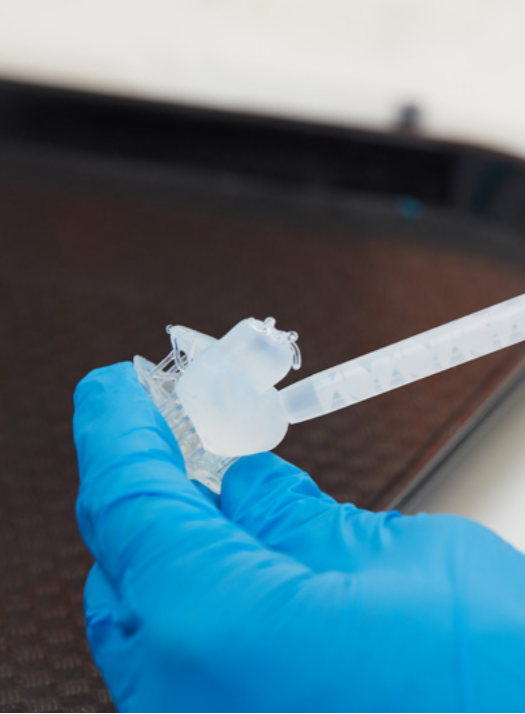
Fig. 16: Injecting the printed shell with BioPor® AB 40 Shore silicone by Dreve.
