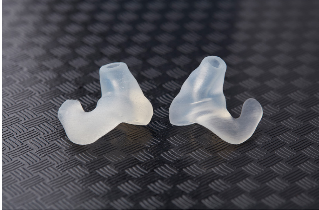
Fig. 17: The ear mold on the left was post-cured in a Form Cure, without pressure. Tiny bubbles throughout the silicone give the ear mold a slightly opaque appearance. The ear mold on the right was pressurized while the silicone cured, so there are no bubbles in the ear mold.
