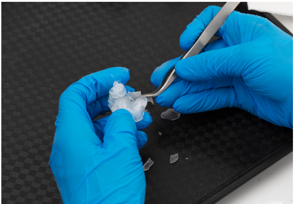
Fig. 19: Cracking and removing the shell from the ear mold.
