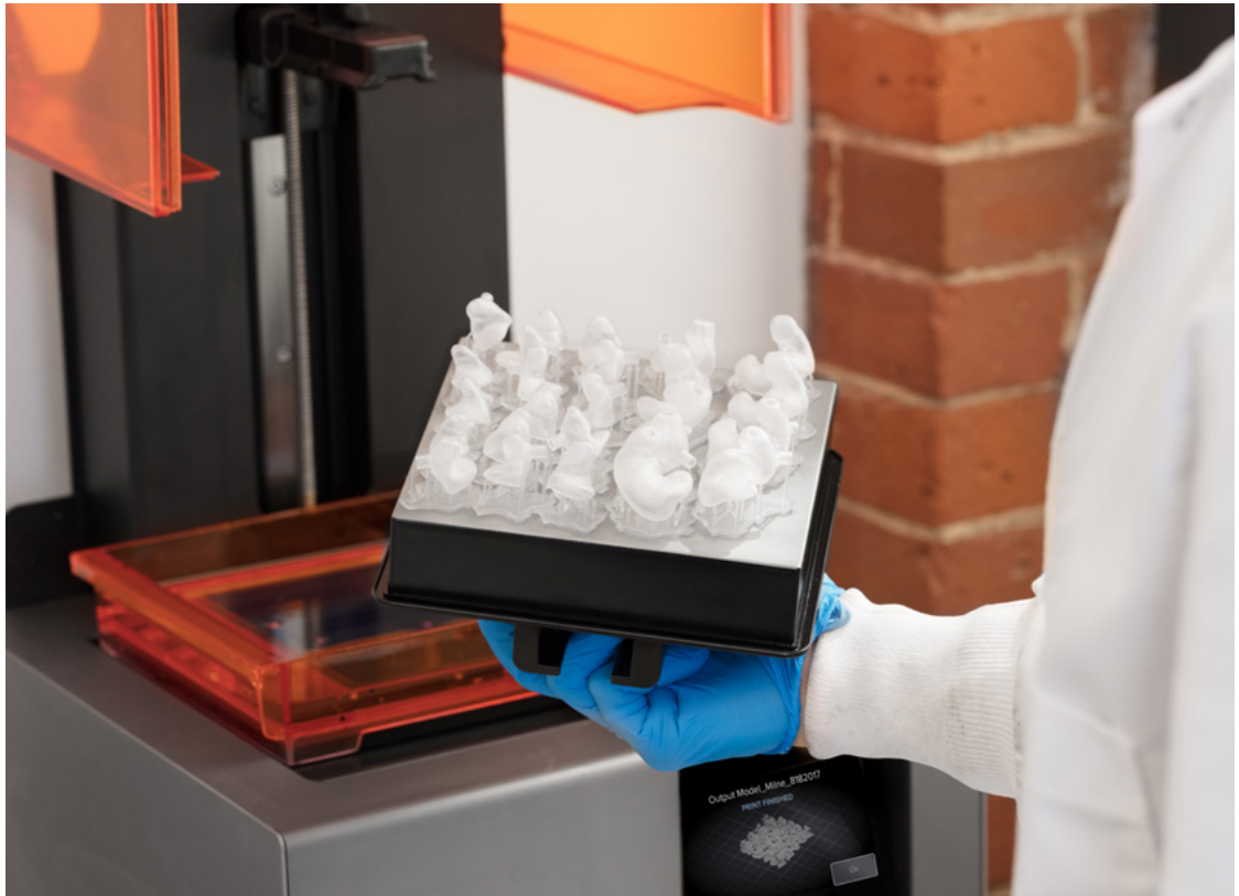
Fig. 12: This full build platform of ear mold shells printed in about 3.5 hours at 100 micron layers.
