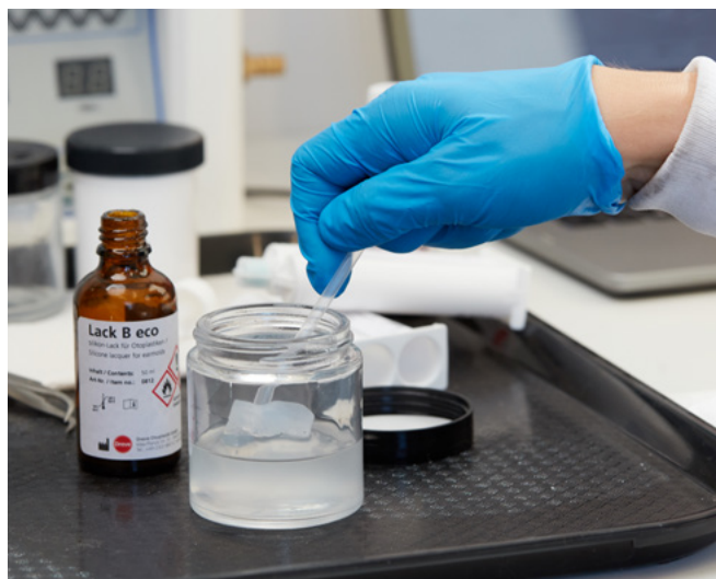
Fig. 21: Coating the silicone in Lack B eco finishing lacquer by Dreve.
