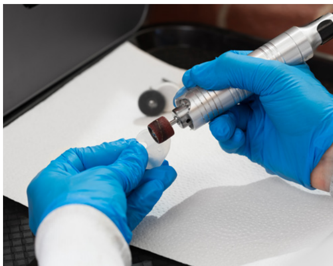
Fig. 20: Finishing the silicone ear mold using a medium grit sandpaper on a flex shaft dremel.
