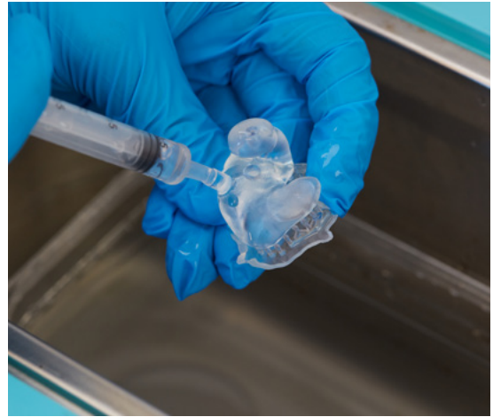
Fig. 14: Injecting the print with IPA to remove any uncured resin.
