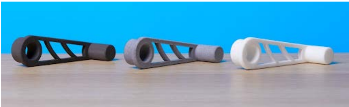
The crank handle replacement part, printed on an in-house Fuse 1+ 30W printer (left), and ordered from a service bureau with an MJF (HP) printer (center), and an SLS (EOS) printer (right).
