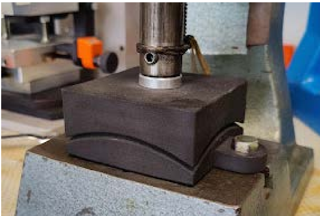
A manufacturing tool printed on the Fuse 1 SLS 3D printer in Nylon 11 Powder for custom eyewear frame pressing.
