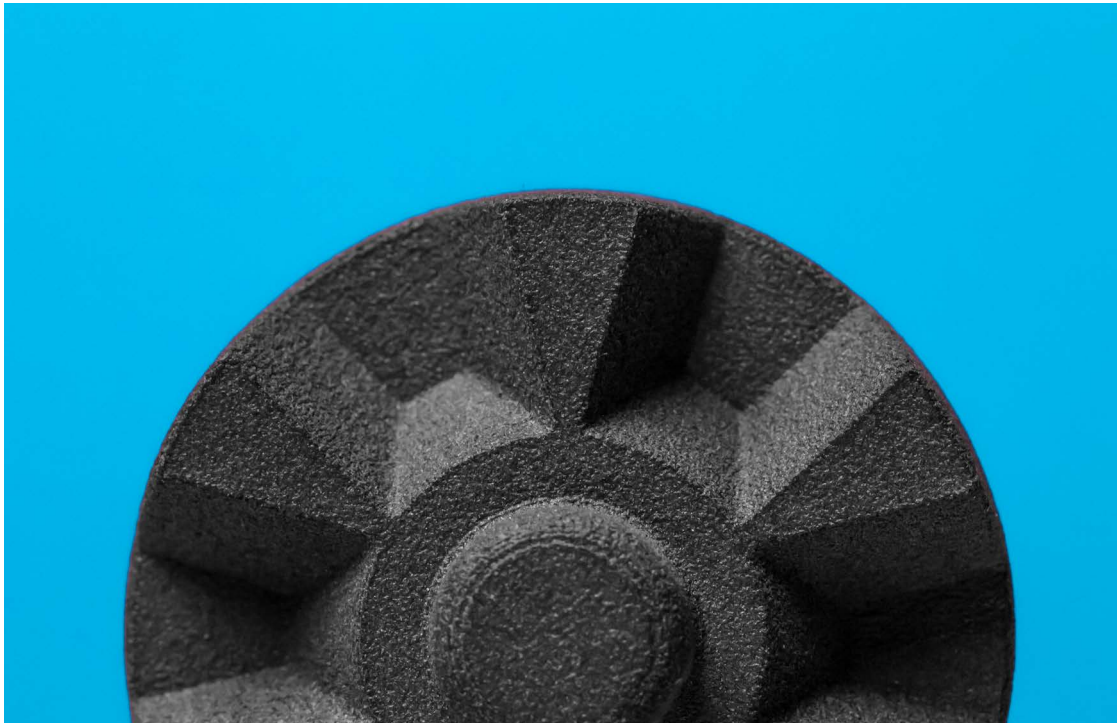
The turntable gear, printed on an in-house Fuse 1+ 30W printer.
