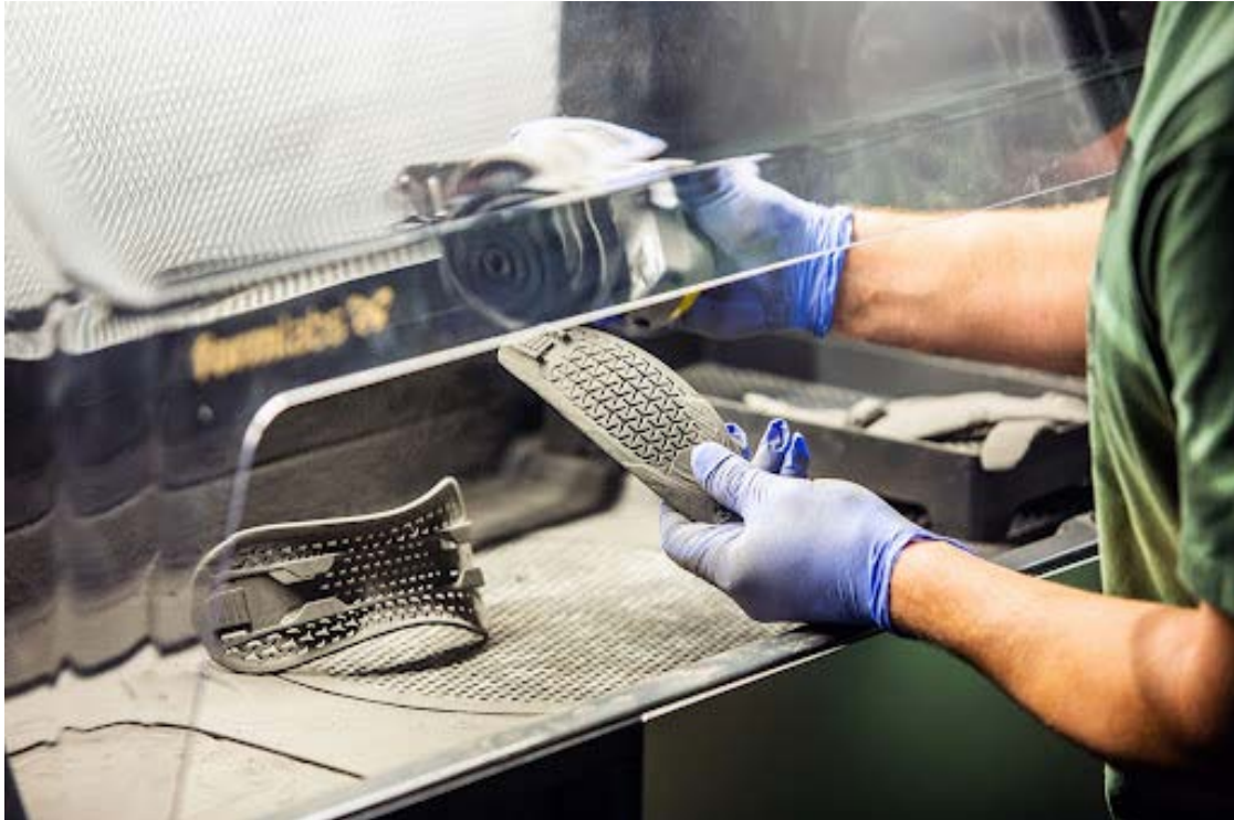
The flexibility and strength of Nylon 12 make it ideal for functional testing of complex assemblies like multi-component snowboard bindings. Photo courtesy of Rome Snowboards.
